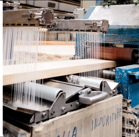
Glueing for face-bonding
